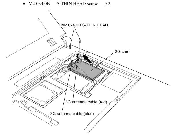
Figure 4-23 Removing the 3G card
